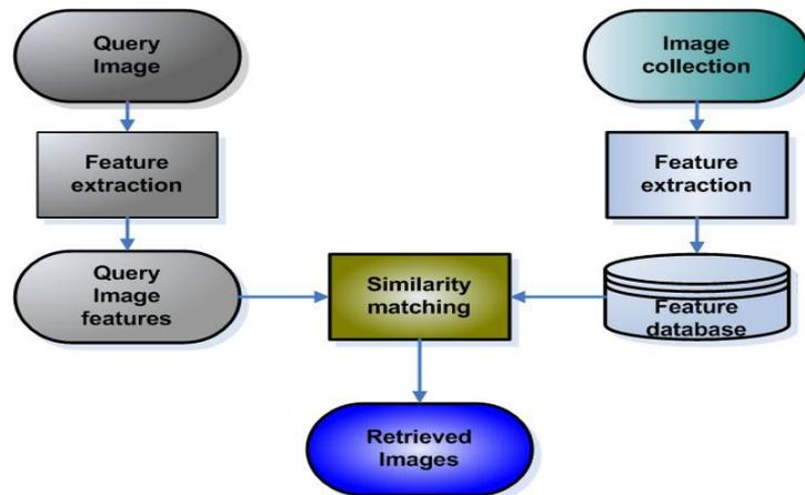
**Fig. 1.** It shows that image retrieved from the large scale database. A single image given as input to that system and then extract the features from the image. Match the features with the features database and display the retrieved images.
